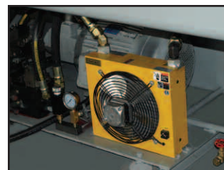
Two Stage Hydraulics with Air Cooler For Long Life
